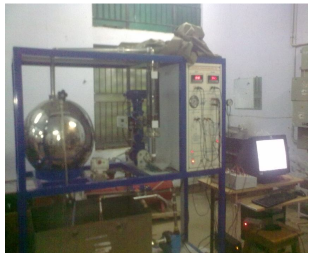
Figures 3 Real time interfacing of VMAT-1 module with Spherical Tank
